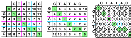
Figures 2a and 2b show the standard dynamic programming distance matrices of the sequences s = \text{GTATC} and t = \text{CTATAC} (using unit cost and penalty +2 for each single insertion/deletion), computed from the upper left to the lower right (Fig. 2a) and from the lower right to the upper left (Fig. 2b). Figure 2c displays the additional-cost matrix , containing the values C_{s,t}[c,d] for each pair of slicing positions (c,d) , e.g. C_{s,t}[2,2] = w_{opt}[\text{CT,GT}] + w_{opt}[\text{ATAC,ATC}] - w_{opt}[\text{CTATAC,GTATC}] = 1 + 2 - 3 = 0 C_{s,t}[4,3] = w_{opt}[\text{CTAT,GTA}] + w_{opt}[\text{AC,TC}] - w_{opt}[\text{CTATAC,GTATC}] = 3 + 1 - 3 = 1 In each matrix, the optimal alignment path is colored green. Its additional-cost matrix entries are, of course, zero.
