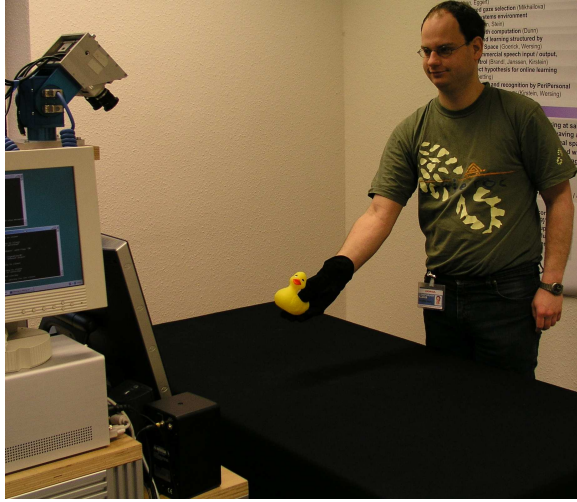
Fig. 3. Experimental setup. Objects are rotated freely by hand in front of a camera. Additionally we use a black glove and show the objects in front of a black table to simplify the foreground-background separation, which is not the focus of this contribution. Using our short-term memory model the recognition system can be trained online to recognize 50 different objects.
